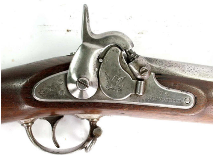
Close up of the Maynard Priming System on the 1855 Springfield
